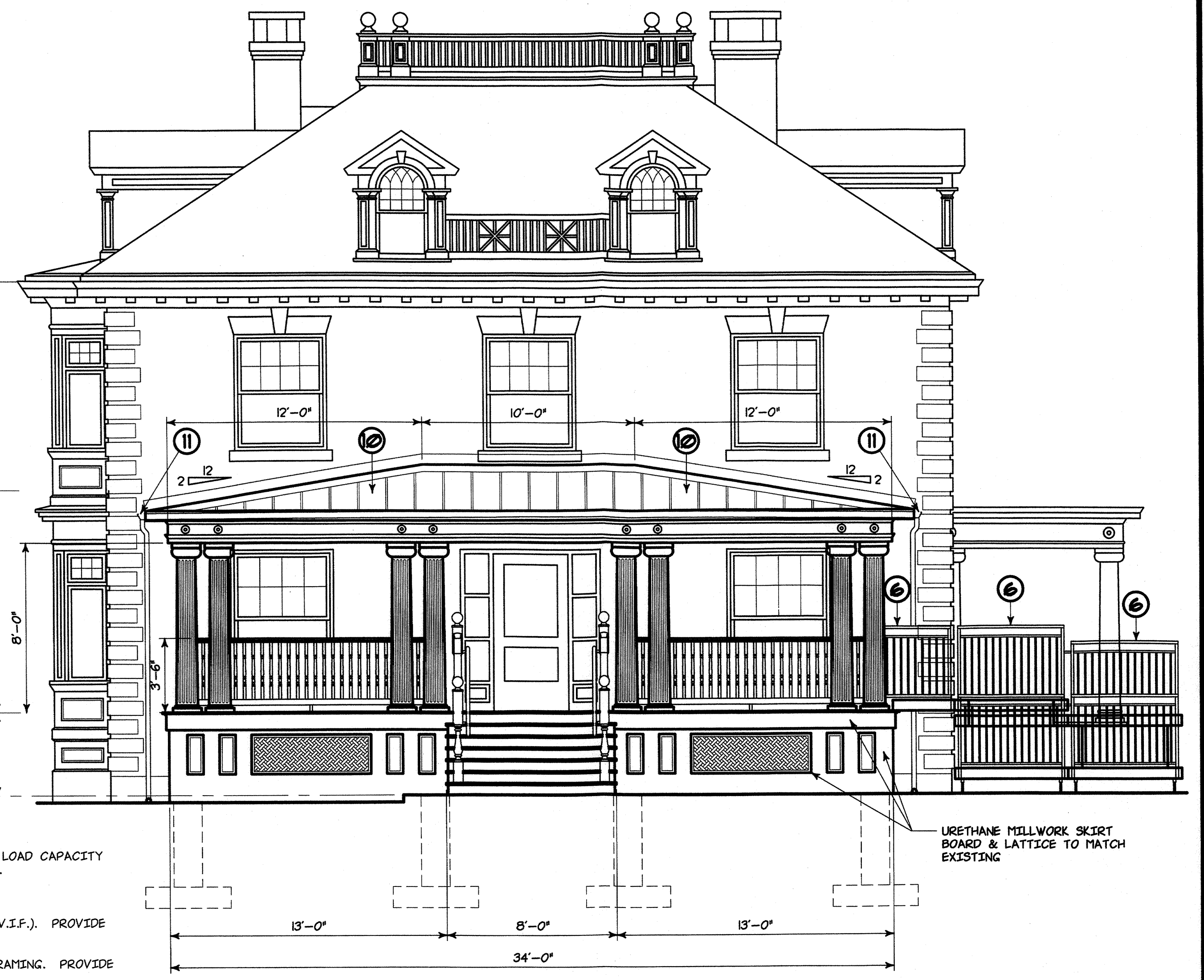
NEW FRONT PORCH - WEST ELEVATION SCALE: 1/4" = 1'-0"
